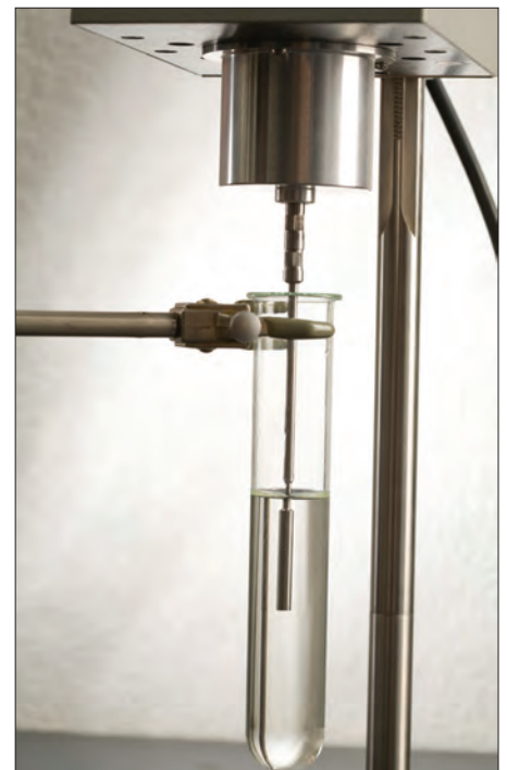
Viscometer device used to determine a liquid's absolute or kinematic viscosity.
