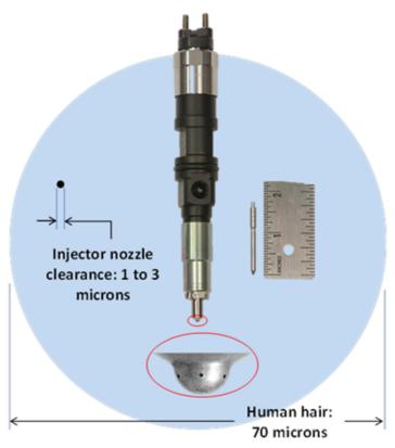
The small clearances of HPCR injectors are susceptible to internal diesel injector deposits that interfere with injector needle actuation. This illustration demonstrates the size of these clearances compared to the diameter of a human hair.
