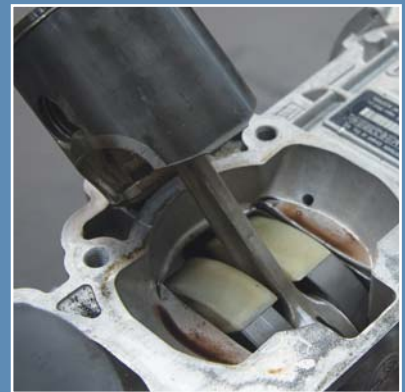
The pistons suffered only minor scuffing.
