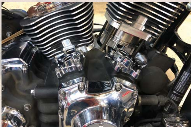
ENGINE REBUILT - Dealer Todd Bleecker ran AMSOIL lubes in his 2011 Harley-Davidson Street Glide with the factory 103 c.i. cylinders for more than 60,000 miles before he rebuilt it with a 110 c.i. big bore kit.
