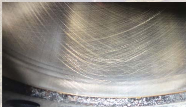
CROSS HATCHING STILL VISIBLE - This photo shows the like-new condition of the cylinders after more than 67,000 miles with AMSOIL 20W-50 Synthetic V-Twin Motorcycle Oil. The obvious cross hatching visible on these well-used cylinders can be attributed to the wear protection properties of AMSOIL synthetic motorcycle oil.
