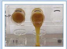
Pour Point is the physical measurement of an oil's fluidity at cold temperatures and refers to the lowest temperature at which the oil maintains its ability to flow. Lower numbers indicate better coldweather wear protection.
