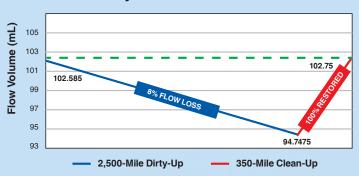
P.i. restored fuel injectors to a 100 percent flow rate after one tank of fuel.
