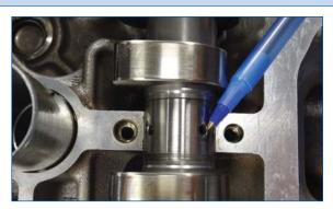
Conventional oils thicken when the mercury drops. Cold, thick oil can fail to flow through the tiny oil passages throughout your engine, like the ones shown here in the camshaft, leading to accelerated wear.
