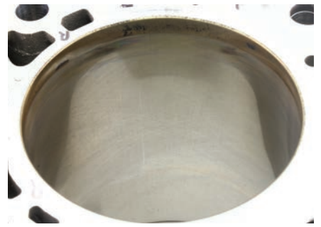
Cylinders are exceptionally clean and well-protected with cross-hatching still visible.
